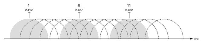
From the results of an RF site survey, you can determine which of the channels the Wi-Fi network is using. With this information, you can see which of the SALLIS channels will be least affected by the Wi-Fi network. The diagram below shows that channels 11, 14, 15, 19, 20, 23, 24, 25 and 26 are the least likely to incur interference from the Wi-Fi network, so these would be the most effective channels to use for your SALLIS network.
