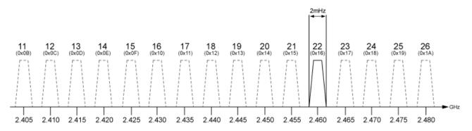
As an example, we can look at how Wi-Fi can affect the operation of SALLIS when it is operating on the same 2.4GHz band. Wi-Fi generally operates on a standard of the IEEE 802.11 communication protocol divided into 14 channels, each occupying 22MHz of bandwidth from 2412MHz to 2484MHz.
